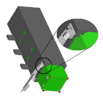
P-POD Deployer with Rail Detail
